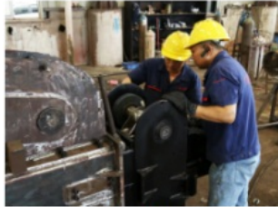
Assemble Precision assembly and tack welding of boom parts.
