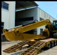
long reach boom
