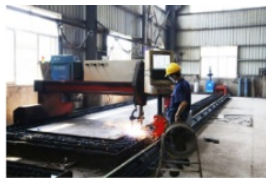
CNC cutting High precision CNC plasma cutting for steel plate blanking
