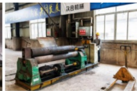
Bending Steel plate bending with large bending machine
