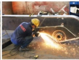
Polishing Grinding and polishing of weld seams and surfaces.
