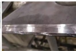
Edge milling Edge milling and beveling for welding preparation
