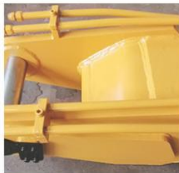
Three Layers with Four Passes Welding
