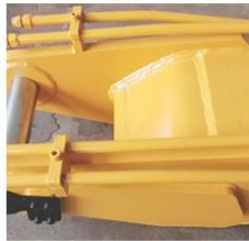
Three Layers with Four Passes Welding
