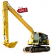
Long Reach Boom
