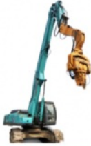
Pile Driving Arm
