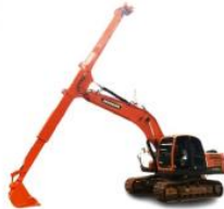
Two-Section Telescopic Arm
