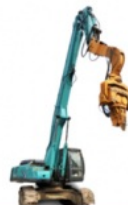
Pile Driving Arm
