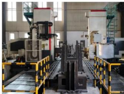
Large double-sided boring machine
