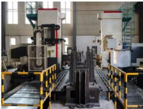
Large double-sided boring machine
