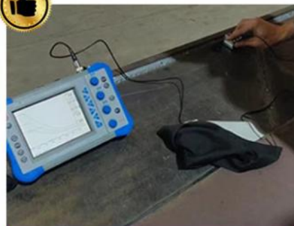
Weld Bead Testing
