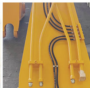
Centralized lubrication system
