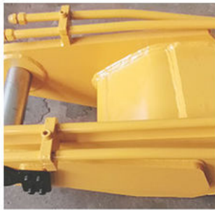
Three Layers with Four Passes Welding
