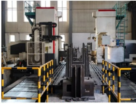
Large double-sided floor boring machine
