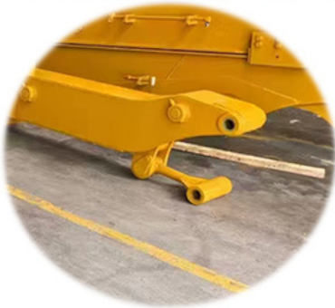
The front end is designed to be curved, greater digging force
