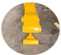
The pivot end is reinforced with multiple layers to withstand greater excavation forces
