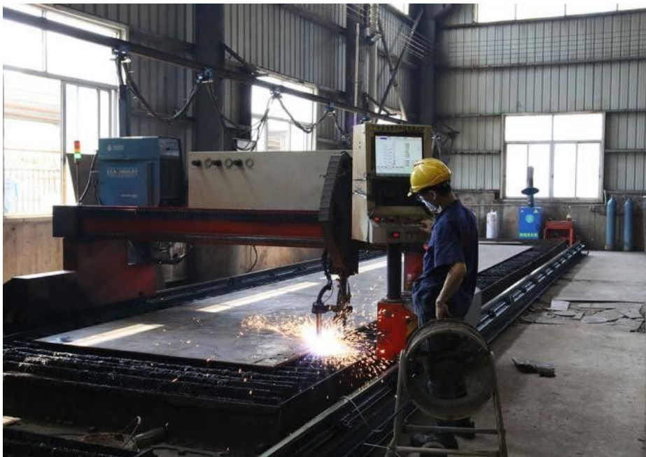
3. Beveling: Every steel is under beveling which ensure high quality welding. Ensure the depth of penetration and the high quality of welds of each set of excavator telescopic arm
