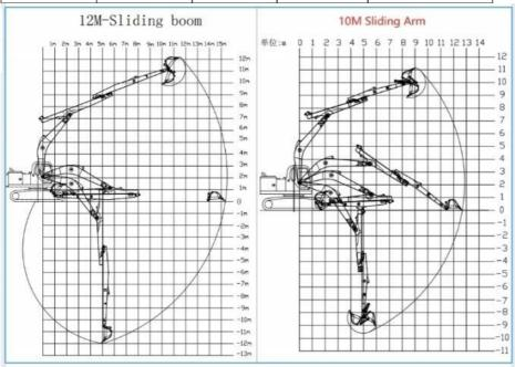
Details of one set of Telescopic Arm telescopic Boom Arm:
