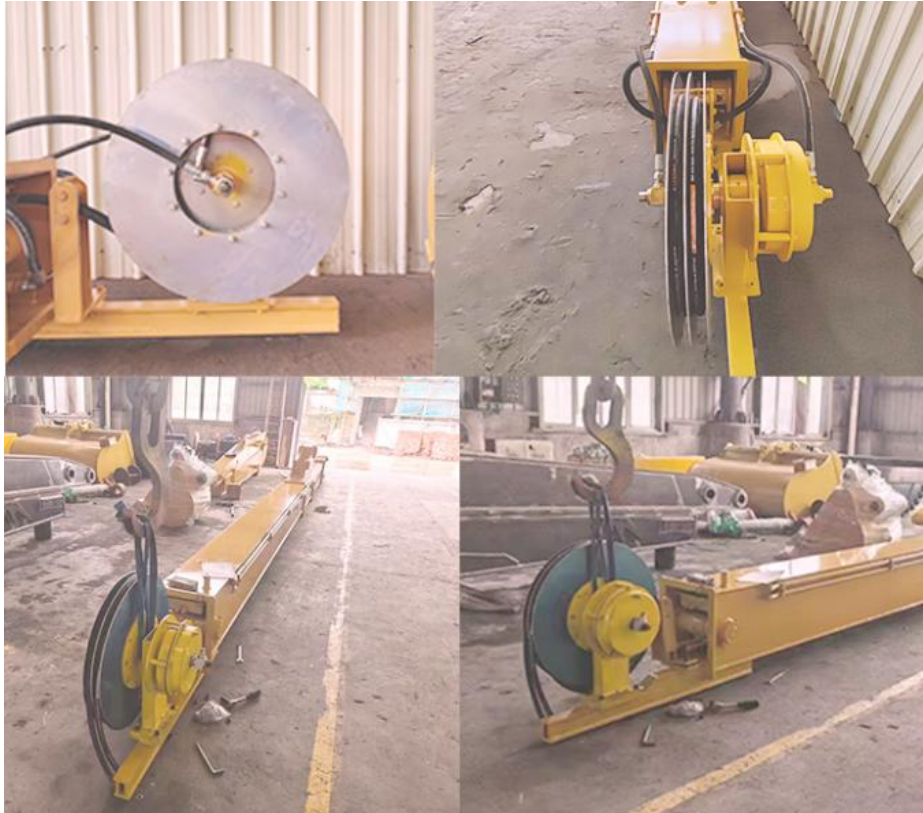
The reel adopts enlarged spring piece
