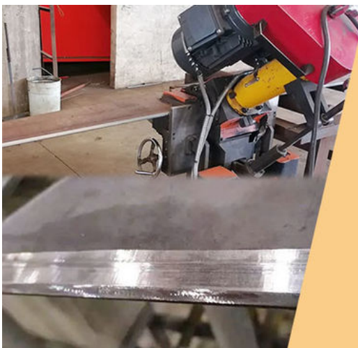
Beveling Machine Every board will be beveled before being welded which enhances the weld bead
