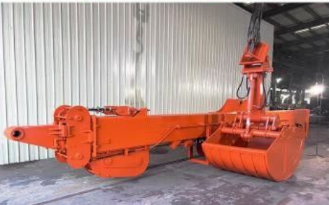
Production details of one set of telescopic arm for excavator:
