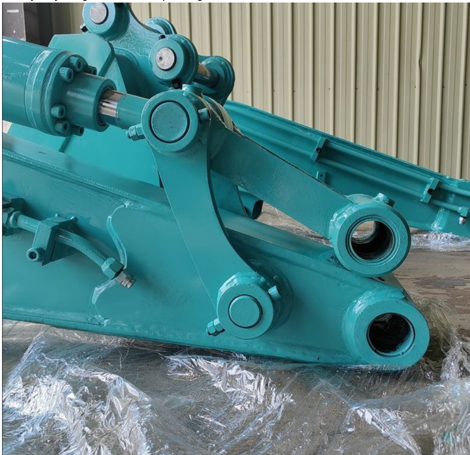
Details of one set of excavator shorten arm: *heavy duty *longer service life-span *high effective
