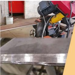
Beveling Machine Every board will be beveled before being welded which enhances the weld bead
