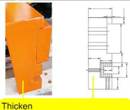
Reduce cracking and failure rate
