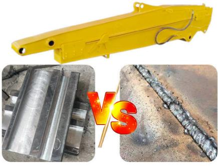
Cut from one plate stronger avoid deformation Welded together Xeasy to crack
