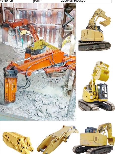
Detail introduction of tunnel arm and boom for excavator:
