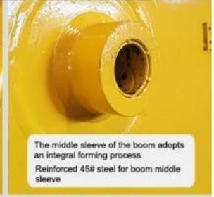
The middle sleeve of the boom adopts an integral forming process
