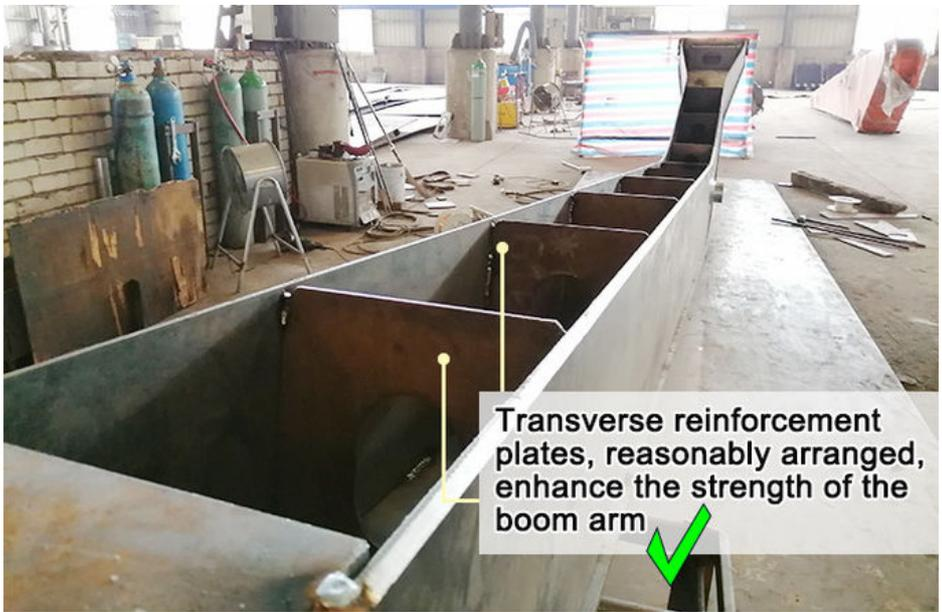
Transverse reinforcement plates, reasonably arranged, enhance the strength of the boom arm
