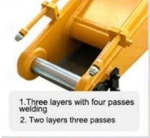
1. Three layers with four passes welding
