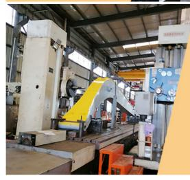
Large floor-standing double-sided boring machine Higher accuracy
