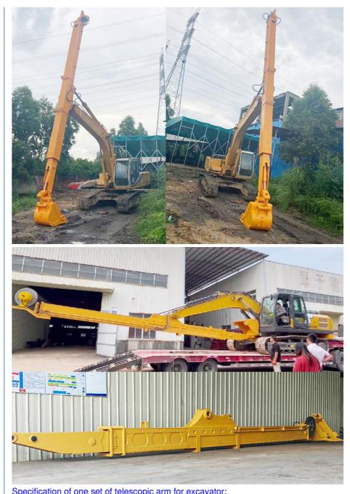
Specification of one set of telescopic arm for excavator: One set of excavator long reach arm include: One telescopic boom, one Bucket, one Bucket Cylinder, One set of Lickage, other accessories
