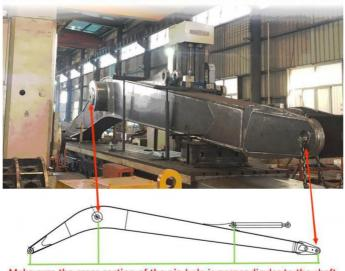
Make sure the cross section of the pin hole is perpendicular to the shaft.
