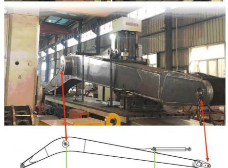
Make sure the cross section of the pin hole is perpendicular to the shaft.
