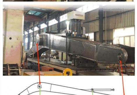
Make sure the cross section of the pin hole is perpendicular to the shaft.
