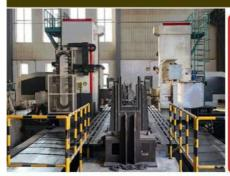
After the excavator boom and arm are assembled, the pins on the boom are drilled to ensure that the pins on the boom are parallel to each other and the cross section of the pin hole is perpendicular to the pin. The double -sided boring machine of the boom makes the hole position more accurate and the quality higher.
